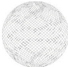
Orbitor 4 nozzle spray pattern
