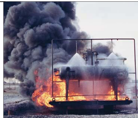
N6 nozzles protect a propane storage tank from fire and explosion.
