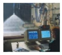
distribution measurement, enabling precise measurement of spray coverage, uniformity, density, and droplet size. **Innovation** is a BETE hallmark, and we are proud that over 60% of the nozzles we ship have been customized to meet the specific needs of a customer. Our new rapid prototype machine speeds development of customized nozzle solutions. We can test a prototype nozzle in our laboratory hours after it was designed for a customer.
